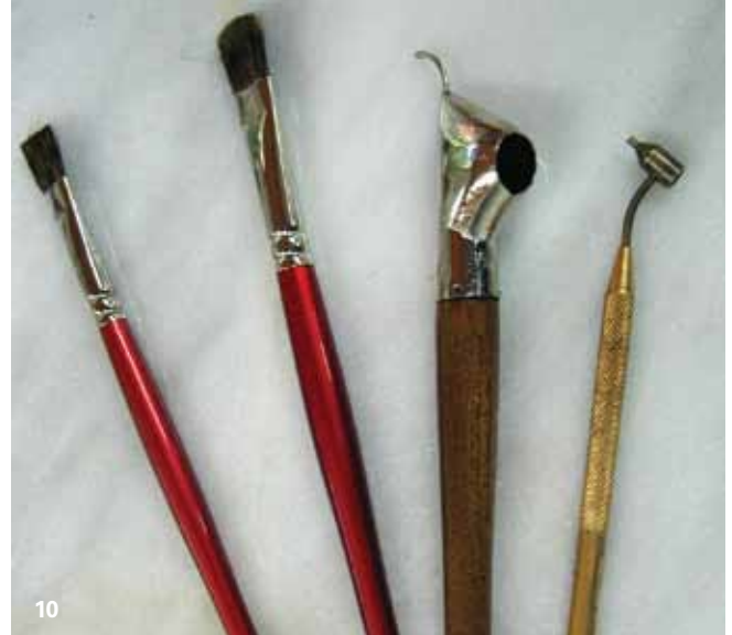
10 From left to right: 3/8-inch and 1/2-inch squirrel-hair flat shaders, tjanting, and gold pen for drawing fine lines.
