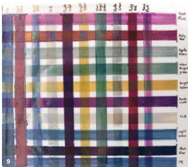
9 Test tile showing the fired results of lusters alone and in layers.
